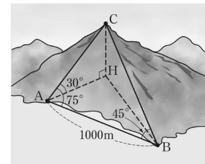
$$\begin{aligned} \angle ACB &= 180^\circ - (\angle ABC + \angle BAC) \\ &= 180^\circ - (45^\circ + 75^\circ) = 60^\circ \end{aligned}$$
